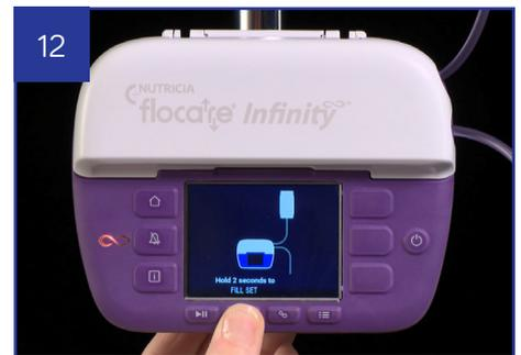
Press and hold the fill set button, after 2 seconds the pump will start
