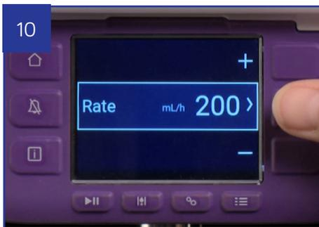
Set rate by pressing the +/- buttons. Press the middle button to confirm
