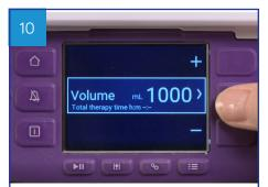
Then select volume and set volume by pressing the +/- buttons. Press the middle button to confirm
