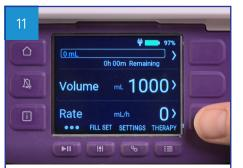
Next select rate and set rate by pressing the +/- buttons. Press the middle button to confirm
